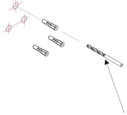
Diameter 8mm masonry drill for walls Diameter 3mm drill for wood/cabinets
